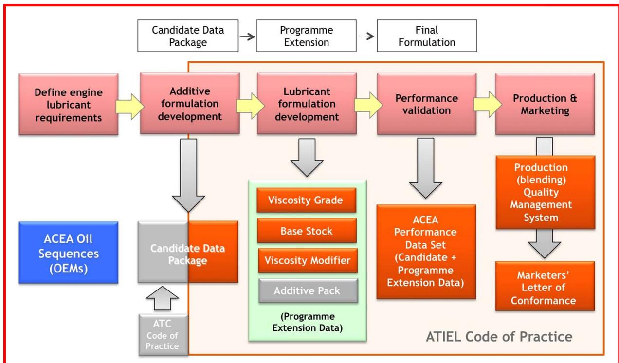
**Figure 1 Steps for developing engine lubricants to meet ACEA Oil Sequences**
