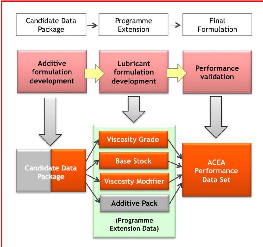
**Figure 2** The derivation of the Programme Extension Data from the Candidate Data Package
