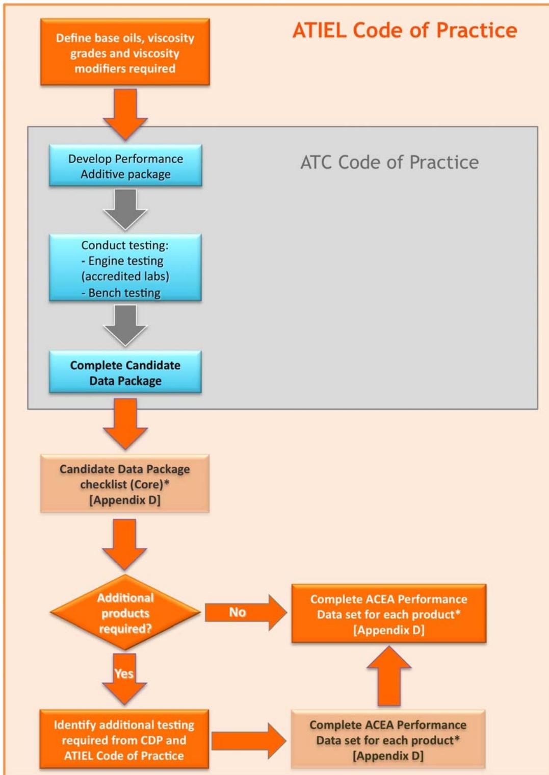
Figure 4 Flow diagram for an EELQMS development programme
